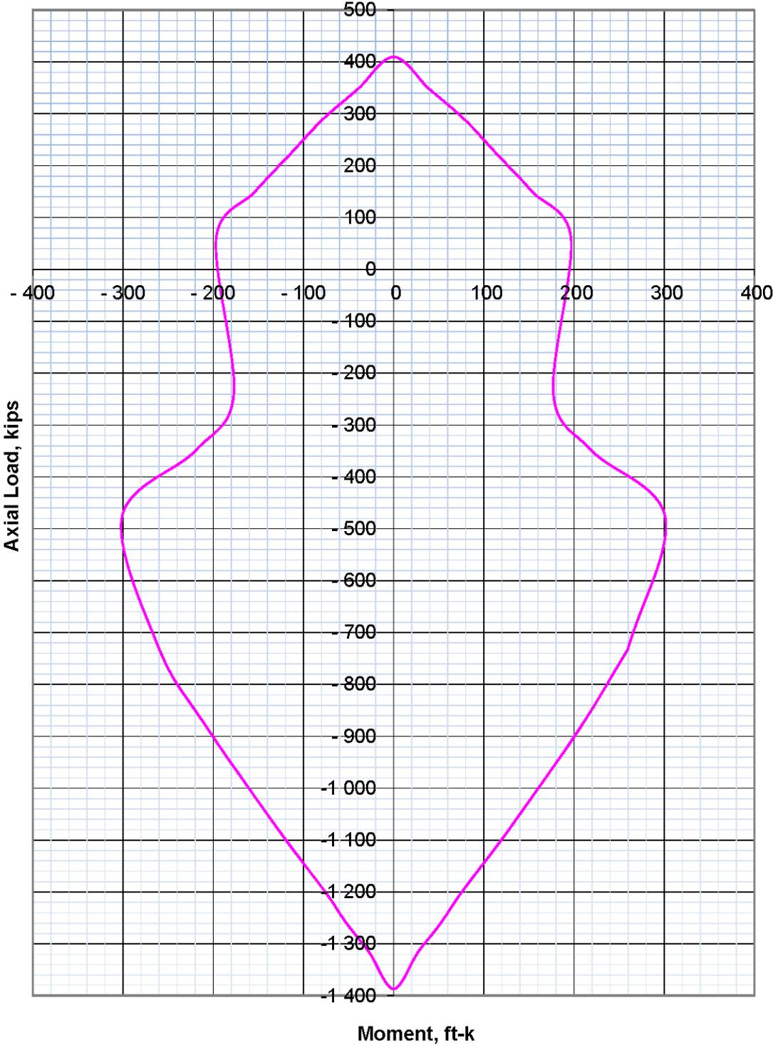
Figure 6. 18-inch Pile Interaction Diagram
