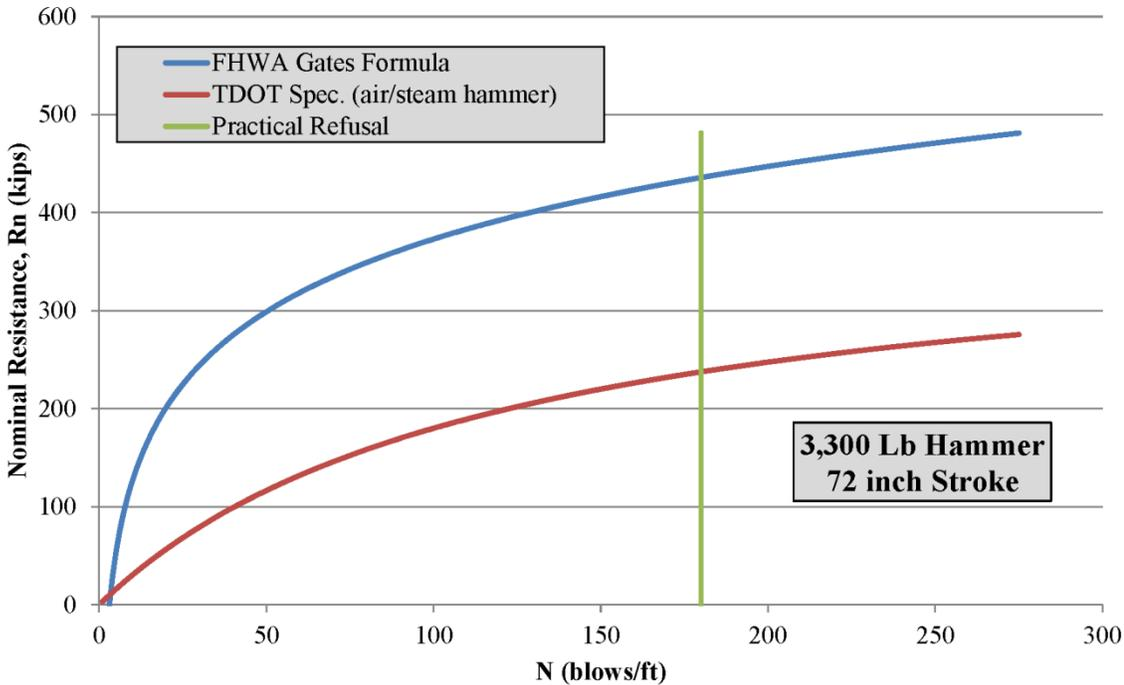
Figure 3. Gates vs. ENR - Case 3
