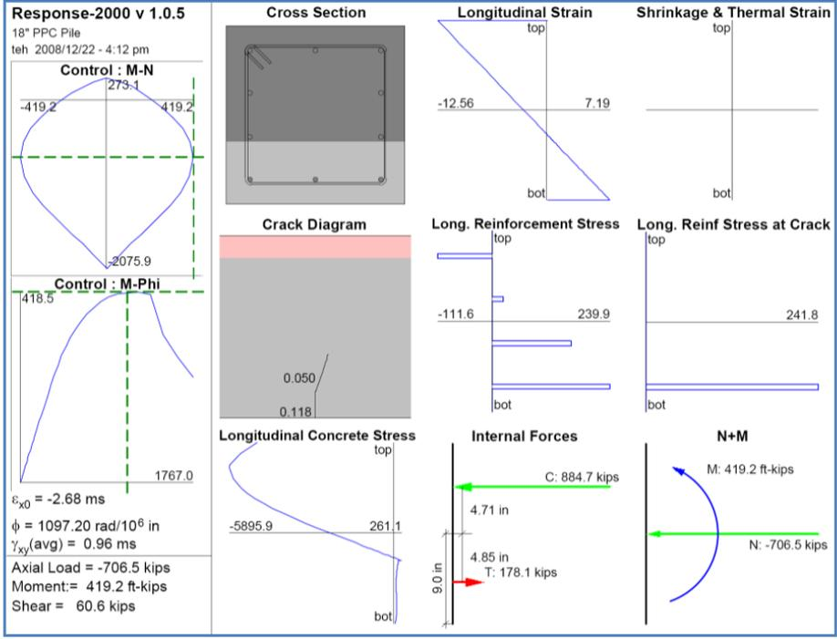
Figure 9. 18-inch Pile Shear Capacity
