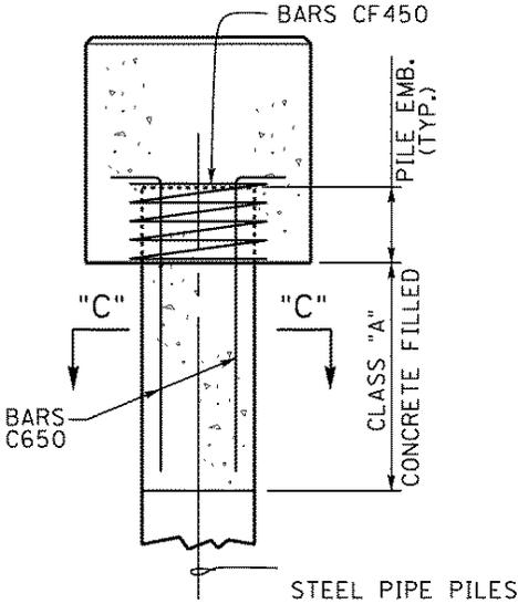
Figure 11. Pipe Pile Connection Details
