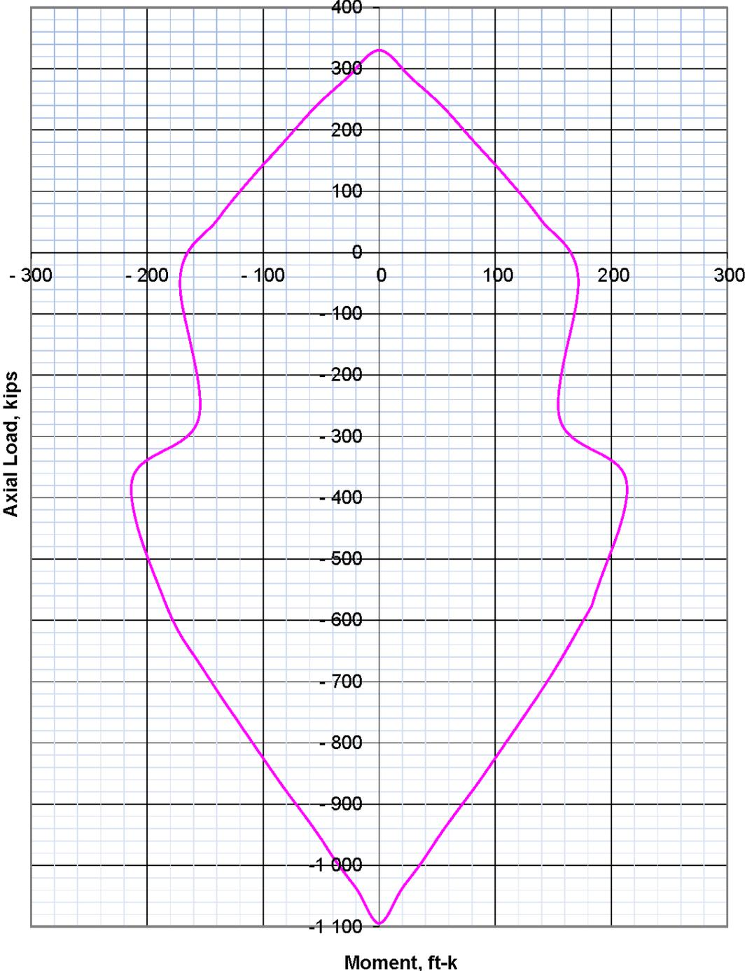
Figure 5. 16-inch Pile Interaction Diagram
