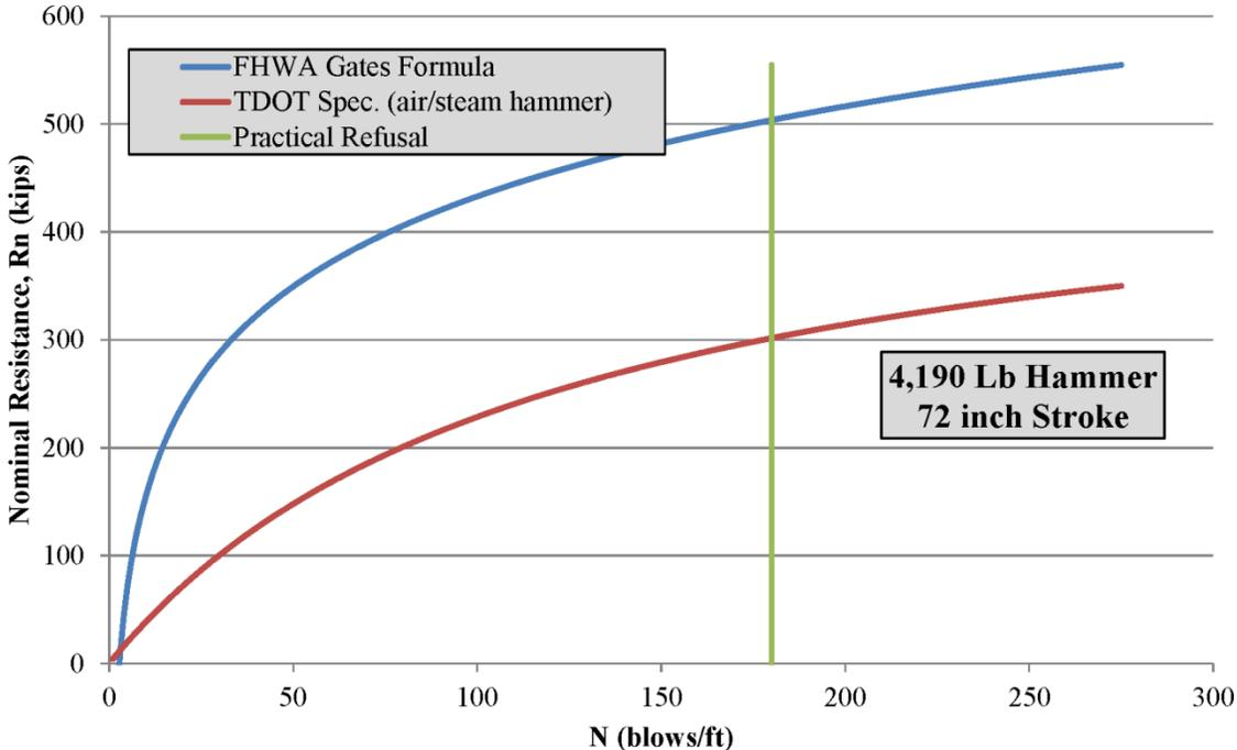
Figure 2. Gates vs. ENR - Case 2
