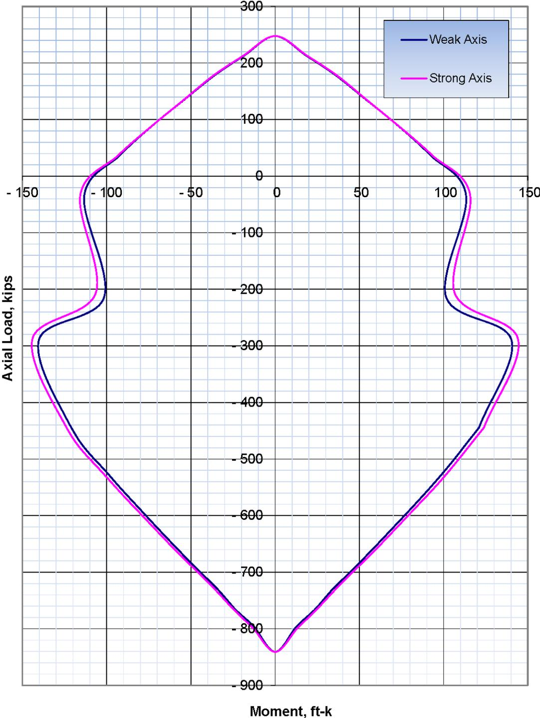
Figure 4. 14-inch Pile Interaction Diagram
