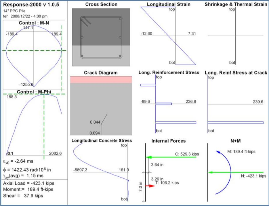
Figure 7. 14-inch Pile Shear Capacity
