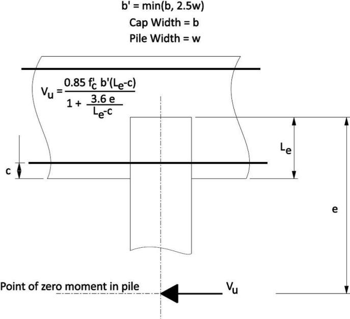
Figure 10. Pile Embedment Requirements
