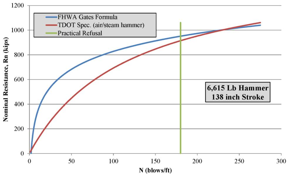
Figure 1. Gates vs. ENR - Case 1
