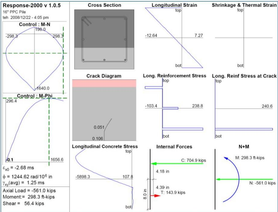
Figure 8. 16-inch Pile Shear Capacity
